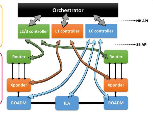
Coriant Groove<sup>™</sup> G30 Network Disaggregation Platform – OLS Solution
